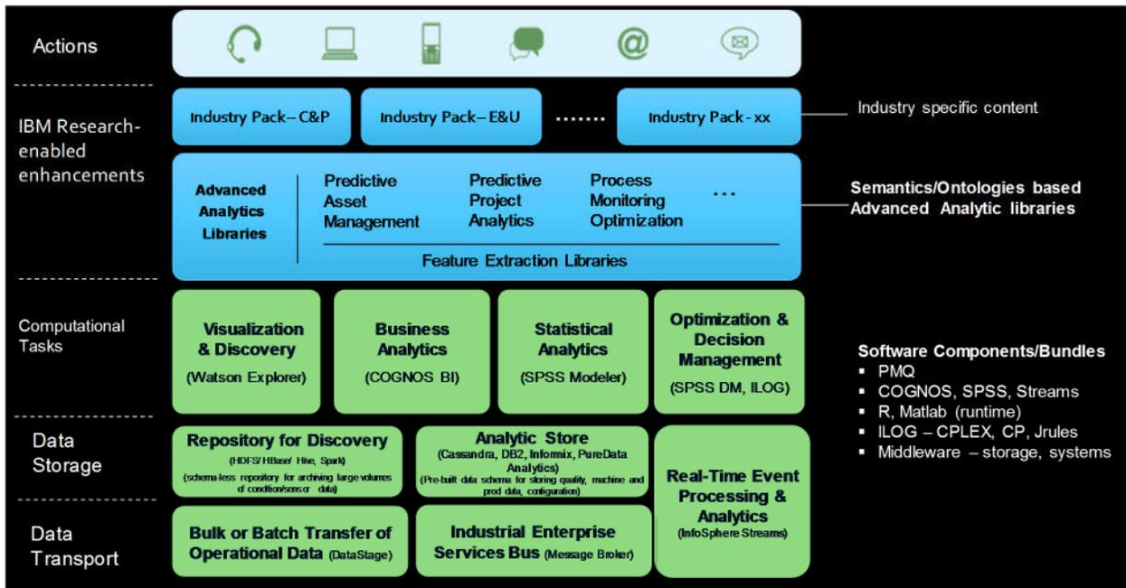
Figure 6: An Architecture for the Semantically defined SROM Analytics Solution
