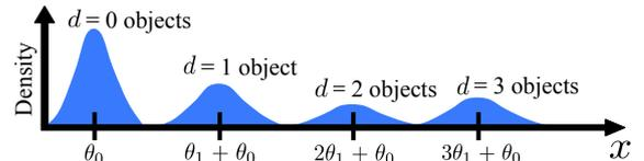
Fig. 1. Illustration of the key idea of mixture-based object counting. The density for a feature  $x$  is represented as a Gaussian mixture which has the sequence of the mean of the feature restricted by the linear function of the count  $d$ .
